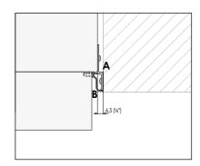
The Lateral Connection Kit (KCLIT/KCLIH/KCLMT/ KCLMH) is supplied on all models (except in the unit with stainless steel sides) and consists of a connection element (A) and a aluminium frame (B).
