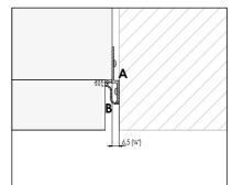
The Lateral Connection Kit (KCLIT/KCLIH/KCLMT/ KCLMH) is supplied on all models (except in the unit with stainless steel sides) and consists of a connection element (A) and a aluminium frame (B).
