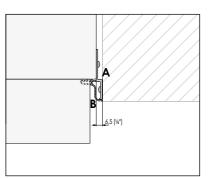
The Lateral Connection Kit (KCLIT/KCLIH/KCLMT/KCLMH) is supplied on all models (except in the unit with stainless steel sides) and consists of a connection element (A) and a aluminium frame (B).
